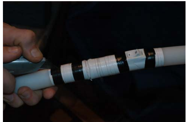
Fig. 2 Cut a 2 nd vertical line to the end of tape.
